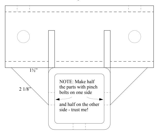
Each piece needs 2 6" pieces of receiver tube and 8  $1.5 \times 1.5 \times 2.125$ " gussets as shown Holes are 1/2" and are to have unplated 1/2-13 nuts welded over them for pinch bolts
