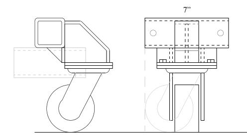
The caster cannot foul against the machine being moved or against an adjacent caster regardless of orientation
